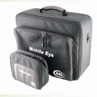
Compact System – all contained in one canvas bag 16 "by 13" by 6" System includes: laptop computer, spectacles with mounted optics and head mounted scene camera (color), modified portable DVCR and EyeVision Software.
